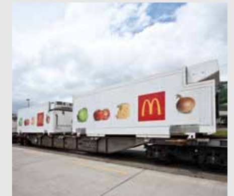
The container is lifted out of the locking system and pushed onto the railway wagon by the Mobiler. The container is placed on the railway wagon and the Mobiler elements are pushed back onto the truck.
