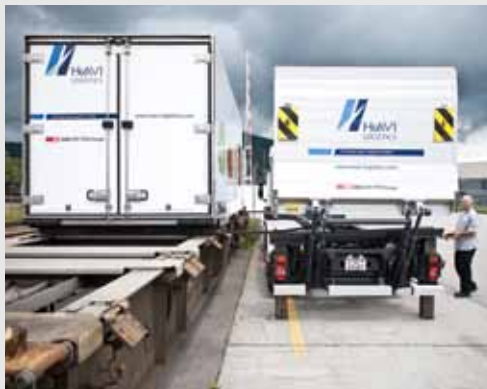
The truck with the mounted Mobiler parks alongside the railway wagon.
