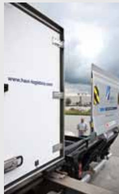
The truck with the mounted Mobiler parks alongside the railway wagon.
