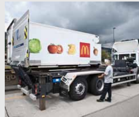
The container is lifted out of the locking system and pushed onto the railway wagon by the Mobiler. The container is placed on the railway wagon and the Mobiler elements are pushed back onto the truck.
